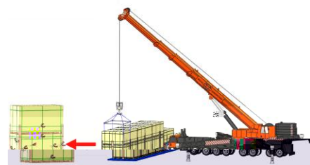
Vertical landscape package unloading with crane
